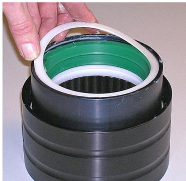
Before you enter the rudder stock, smear some grease on the lips. Don't use too much grease as it shouldn't enter the roller section of the bearing.
