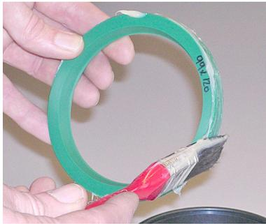
Use a small brush to smear some synthetic grease (we use Castrol Synplex 2, but any winch grease will do the job) on the outside of the seal. You can find the grease in the small plastic bag supplied with the seals.
