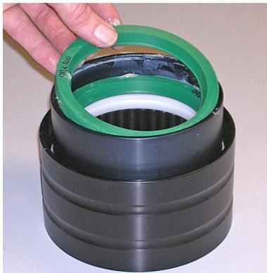
Mount the second seal and fit the delrin clip. This clip will prevent the lip seal from climbing upwards.
